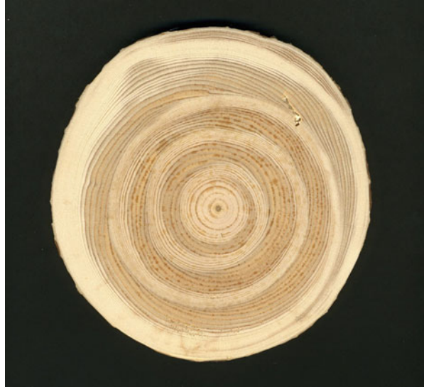
Fig. 1.1 Spiral compression wood in a Scots pine ( Pinus sylvestris L.) stem from a first thinning site in southern Finland. The disk shows a band of compression wood that spirals four times clockwise from the pith towards the cambium. The formation of compression wood began when the tree was 5–6 years old and continued for several decades
