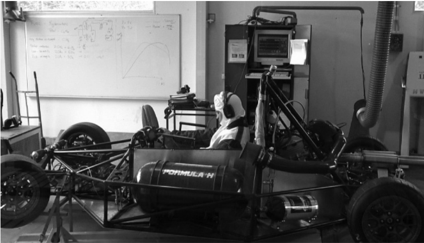
Figure 1.9 Tank assembly of the Formula H racing car, developed by the University of Applied Sciences Ingolstadt and RMIT Melbourne, see [6].
